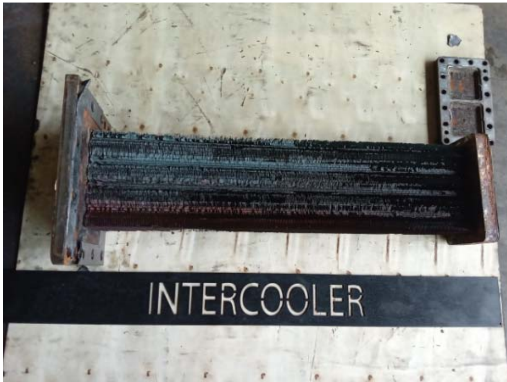
INTERCOOLER BEFORE CLEANING
