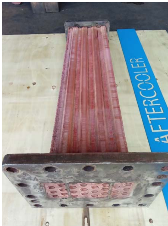
AFTERCOOLER AFTER CLEANING
