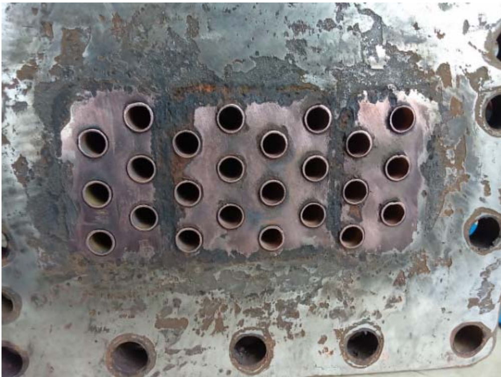
AFTERCOOLER AFTER CLEANING
