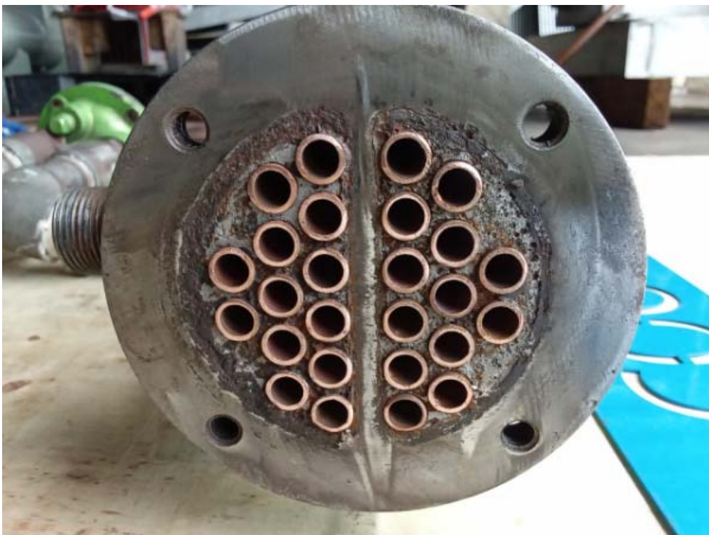
OIL COOLER AFTER CLEANING
