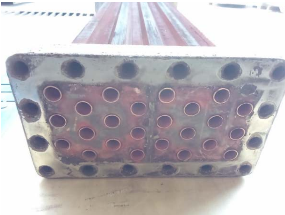
AFTERCOOLER AFTER CLEANING
