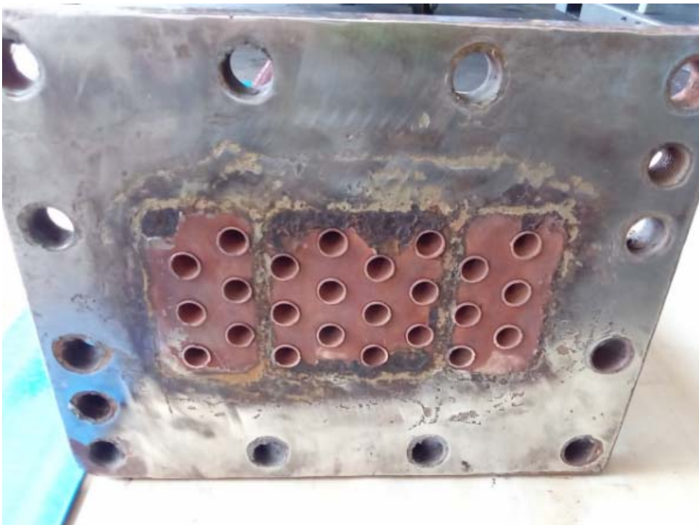
INTERCOOLER AFTER CLEANING
