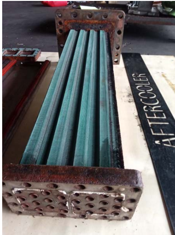
AFTERCOOLER BEFORE CLEANING
