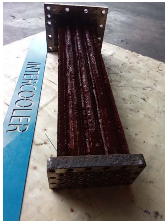
INTERCOOLER AFTER CLEANING
