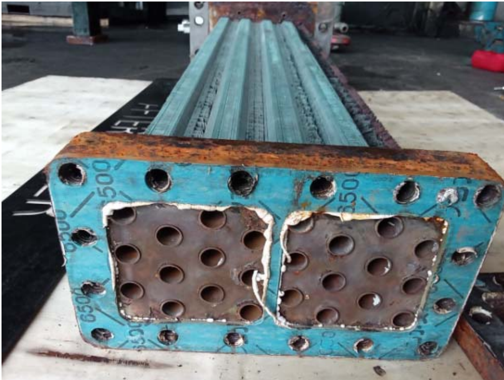
AFTERCOOLER BEFORE CLEANING
