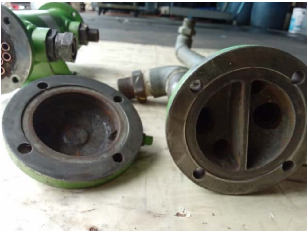
OIL COOLER AFTER CLEANING
