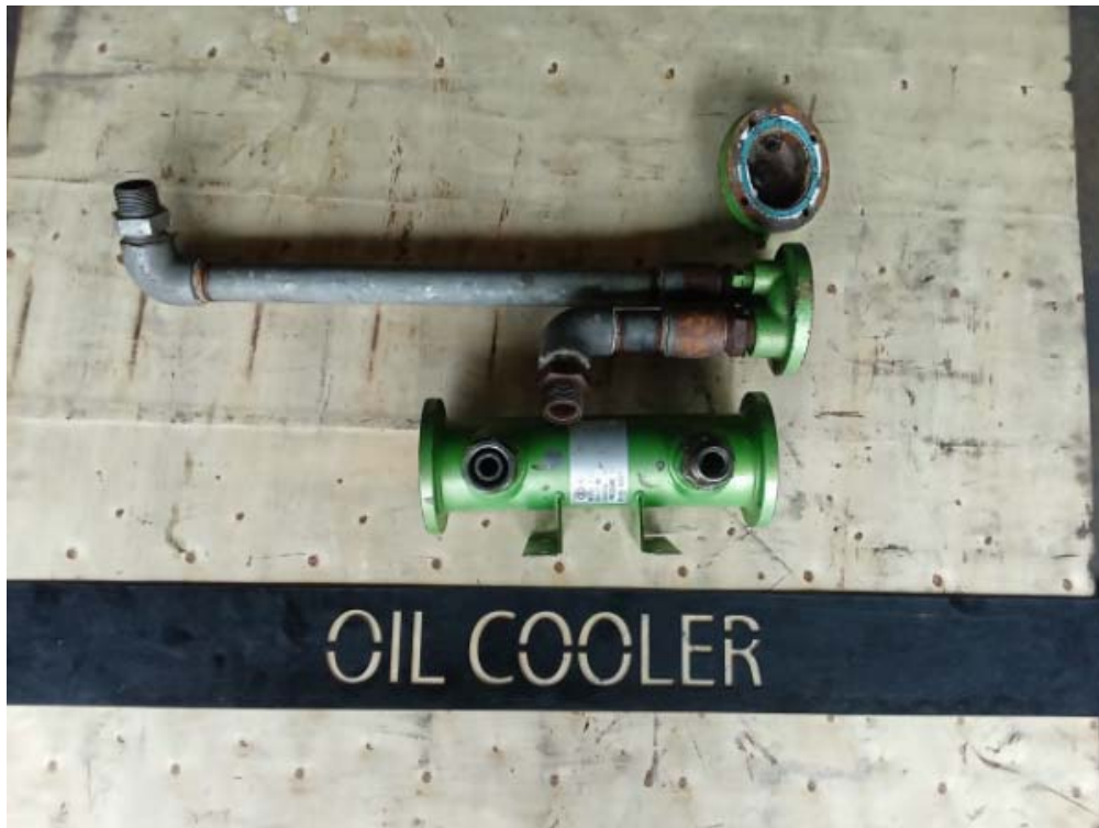
OIL COOLER BEFORE CLEANING
