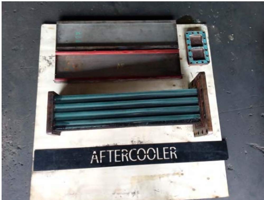
AFTERCOOLER BEFORE CLEANING
