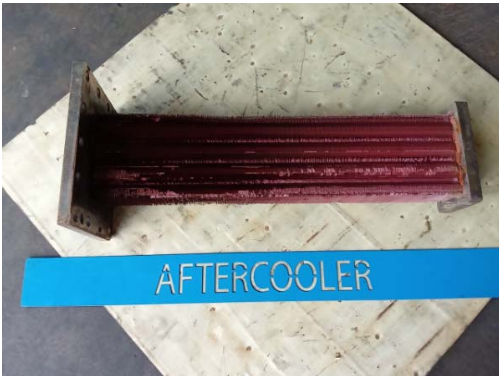
AFTERCOOLER AFTER CLEANING
