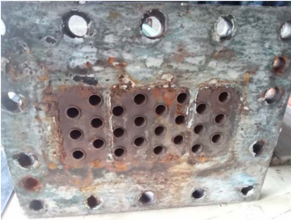
AFTERCOOLER BEFORE CLEANING
