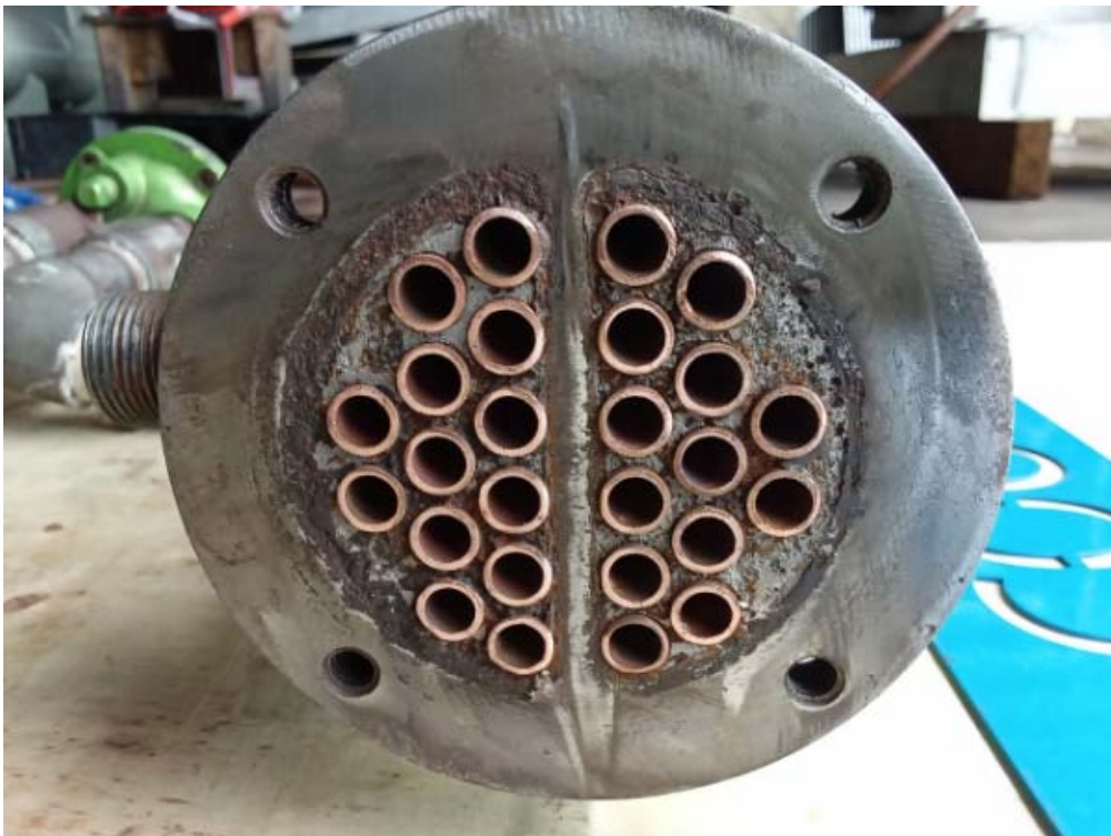
OIL COOLER AFTER CLEANING
