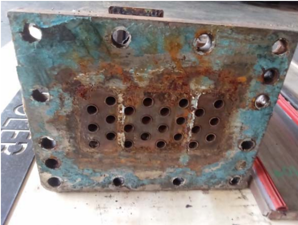
INTERCOOLER BEFORE CLEANING
