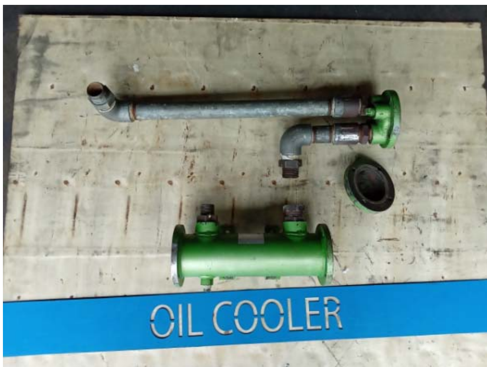
OIL COOLER AFTER CLEANING
