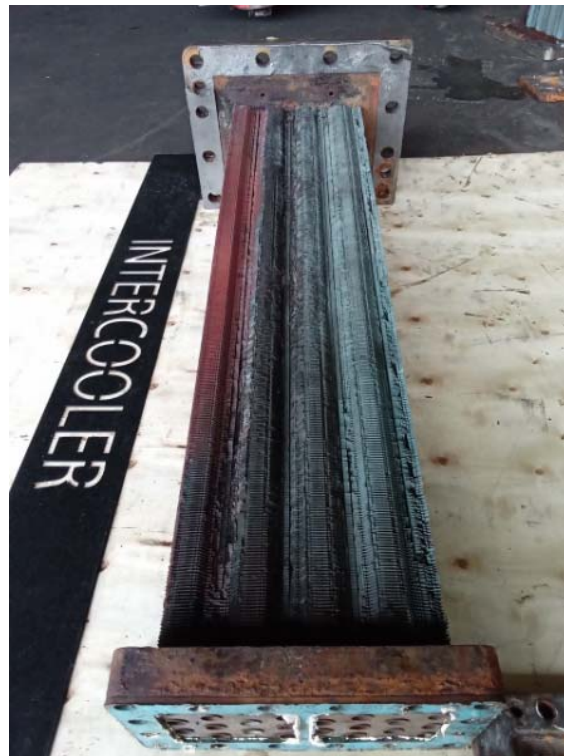
INTERCOOLER BEFORE CLEANING
