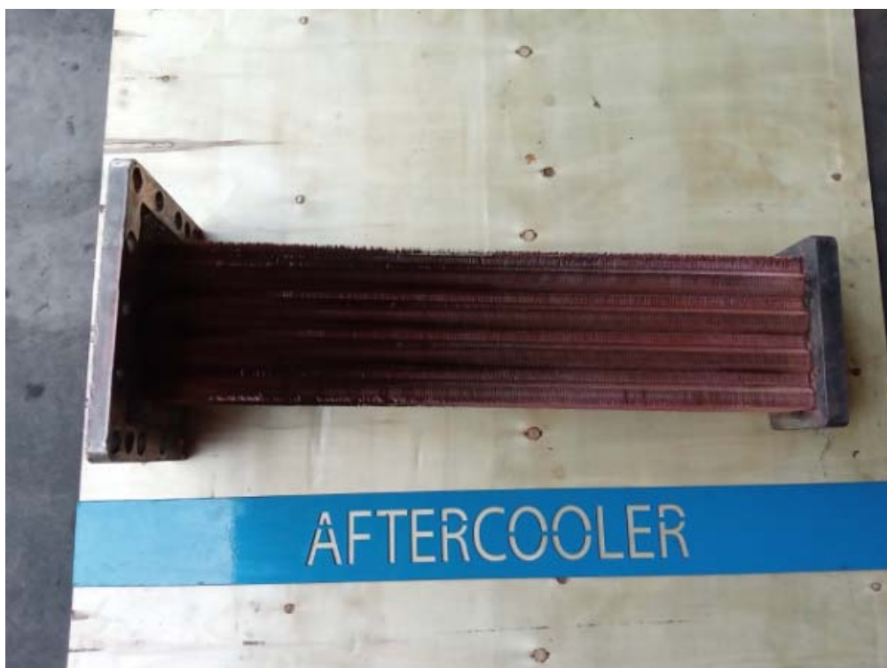
AFTERCOOLER AFTER CLEANING
