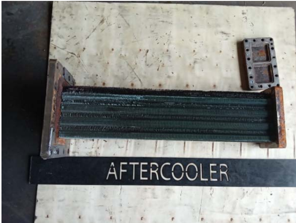
AFTERCOOLER BEFORE CLEANING
